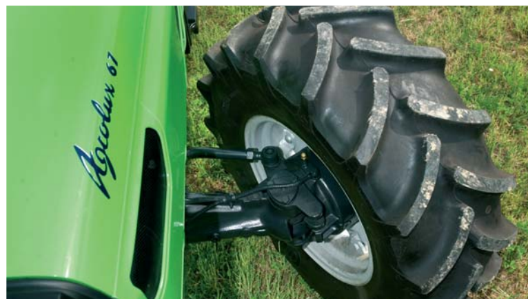
A tight steering angle of 50° provides impressive maneuverability.
